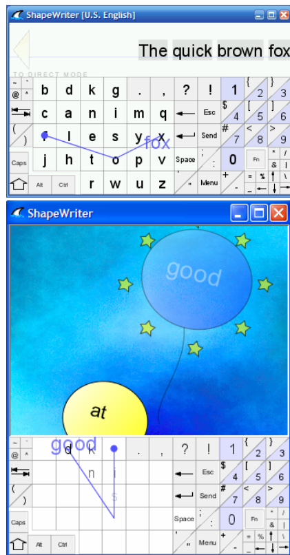
Figure 3. ShapeWriter (top) and the ‘brushing’ training game (bottom). The ideal trace of the recognized sokgraph is displayed on the keyboard.
