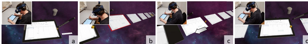
Figure 3: Interacting with multiple sheets using: initially, solely icons indicating the existent of additionally accessible sheets are visible (a). Neighboring sheets are expanded and each sheet the user gazes at is highlighted with a red frame (b). The user taps with his non-dominant hand on the tablet bezel, causing the selected sheet to slide towards the tablet (c), where the user can edit it using the tablet's touchscreen.
