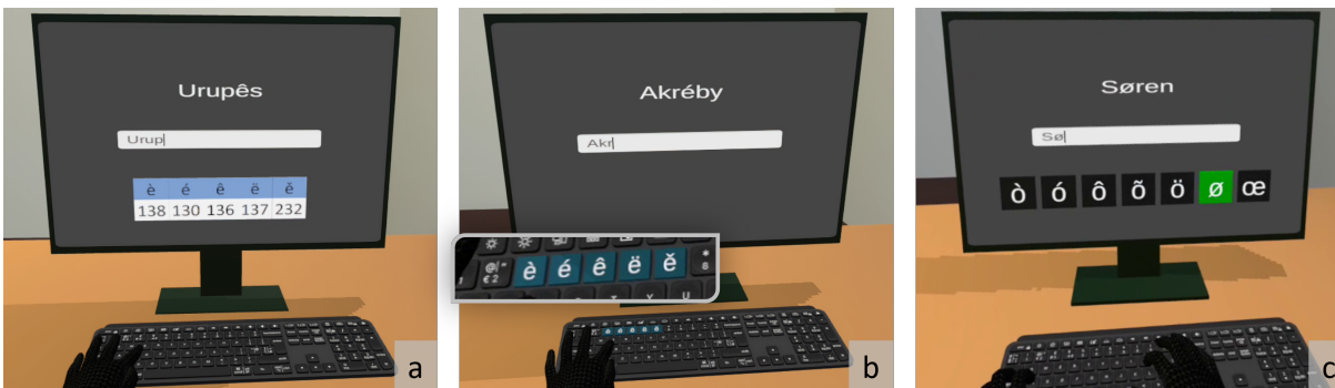
Figure 1: Techniques for entering accented characters in VR: a) BASELINE technique which displays numeric codes for relevant accented characters after pressing a modifier key (Alt) and a base character and then requires the user to enter the respective numeric code; b) RECONFIGURATION technique as presented by Schneider et al. [48] which overlays the accented characters onto the keyboard when pressing a modifier key (Alt) and a base character; c) MULTIMODAL technique which presents the accented characters on the virtual screen while pressing a modifier key (Alt) and a base character and enables the user to select one via eye-gaze and confirm by key press.
