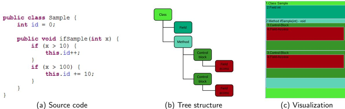
Figure 3. Source code, its tree representation, and its nested tree visualization.
