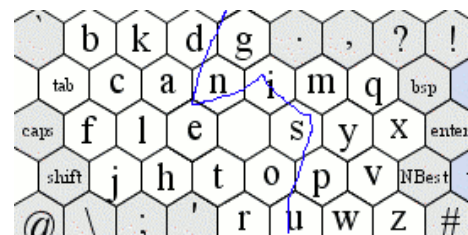
Figure 2: The user is writing “using” on the ATOMIK layout using the SHARK 2 system.
