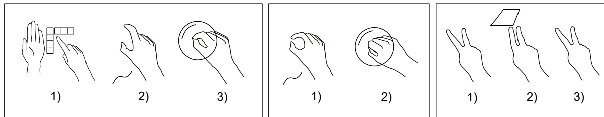
Fig. 1: Illustration of conventional menu-based tool selection and HotGestures. Left) The user selects the sphere primitive tool from the menu, moves their hand to where they want to place the sphere, and then performs a pinch gesture to confirm its placement. Middle) The user moves their hand to where they want to place a sphere primitive, and then performs the sphere HotGesture to place it in a single gesture articulation. Right) The user can modulate the state of the HotGesture to control tool triggering, such as to designate the start and end of a planar cut.
