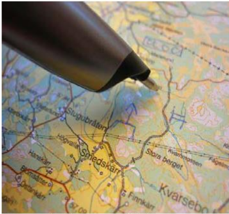
Figure 1: Drawing NATO symbols on a paper map with a digital Aoto pen.
