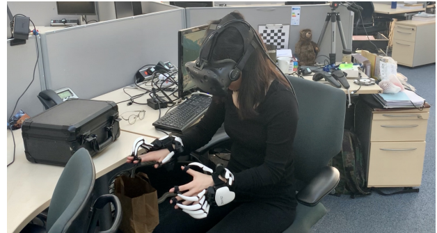
Figure 1: A participant is trying the system with an HTC Vive HMD and Dexmo gloves.
